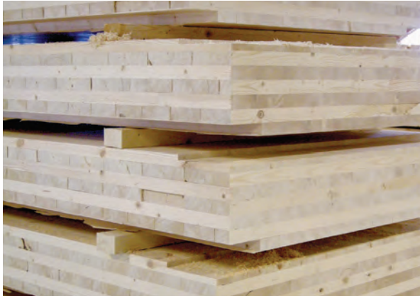
FIGURE 2-3: Lumber CLT (left); SCL CLT (right) Images: FPIinnovations (left); Freres Lumber (right)
